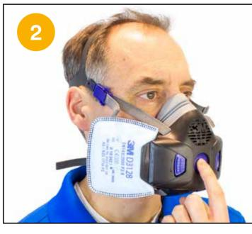
2. Lightly press the seal check button until you feel resistance. Hold the button in this position and inhale gently. If you feel the facepiece collapse slightly and pull closer to your face with no leaks between the face and facepiece, a proper seal has been obtained.
