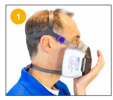
Cover the opening of the exhalation valve cover with your hand and exhale gently. If the facepiece bulges slightly and no air leaks are detected between your face and facepiece, a proper seal has been obtained.
